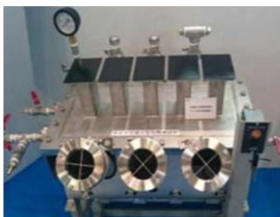
Microwave heating equipment employing GaN amplifier modules as heat sources
