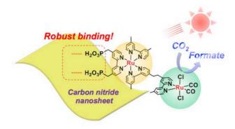
**Figure**. Schematic of solar fuel production by semiconductor photocatalyst Researchers observed robust binding between the ruthenium metal complex and carbon nitride nanosheets under visible light in aqueous solution © *Angew. Chem.*
