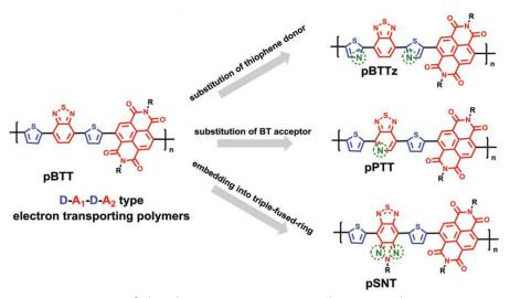
Figure 1. Design of the three n-type semiconducting polymers. By strategic embedding of sp<sup>2</sup>-N atoms in BTT, three different polymers were synthesized and used to fabricate thin-film transistors.
