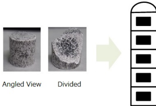
Figure 1 Fabrication of antenna structure using dolomite and ferrosilicon (Left) Actual pellet of dolomite and ferrosilicon. White portion is dolomite rich, and the black portion is ferrosilicon rich. Ferrosilicon is concentrated in the center portion. (Right) Five stacked to form the microwave wavelength (antenna structure).
